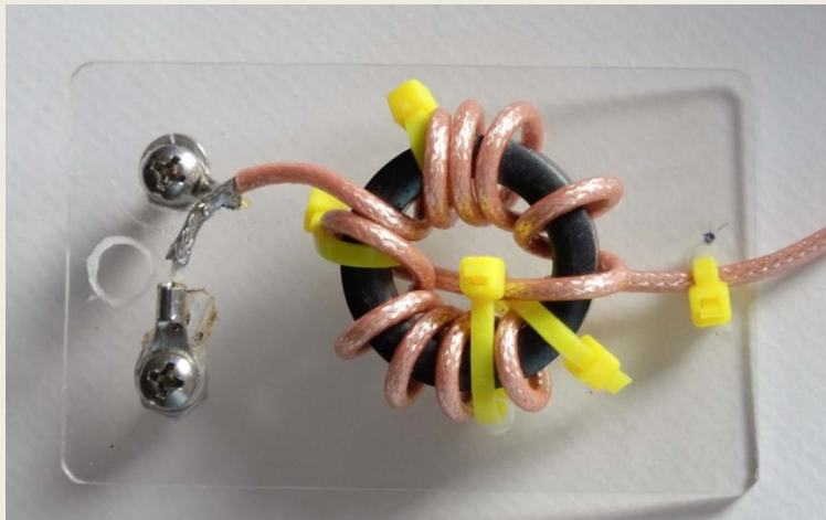
1:1 Balun RG316 Ferrite Core
