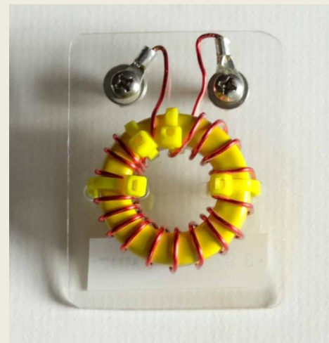
Loading Coil Powdered Iron High Q: 20 m monoband antenna
