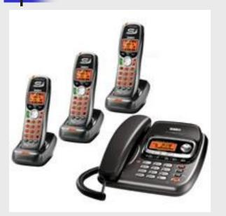
This Uniden model uses frequencyhopping digital spread spectrum mode. Most cheaper models are analog FM and operate base-handset at 5.9GHz but handset-base at 900 MHz. <u>The corded</u> handset in this base replaces the P.O.T.S. for speech to/from handsets.
