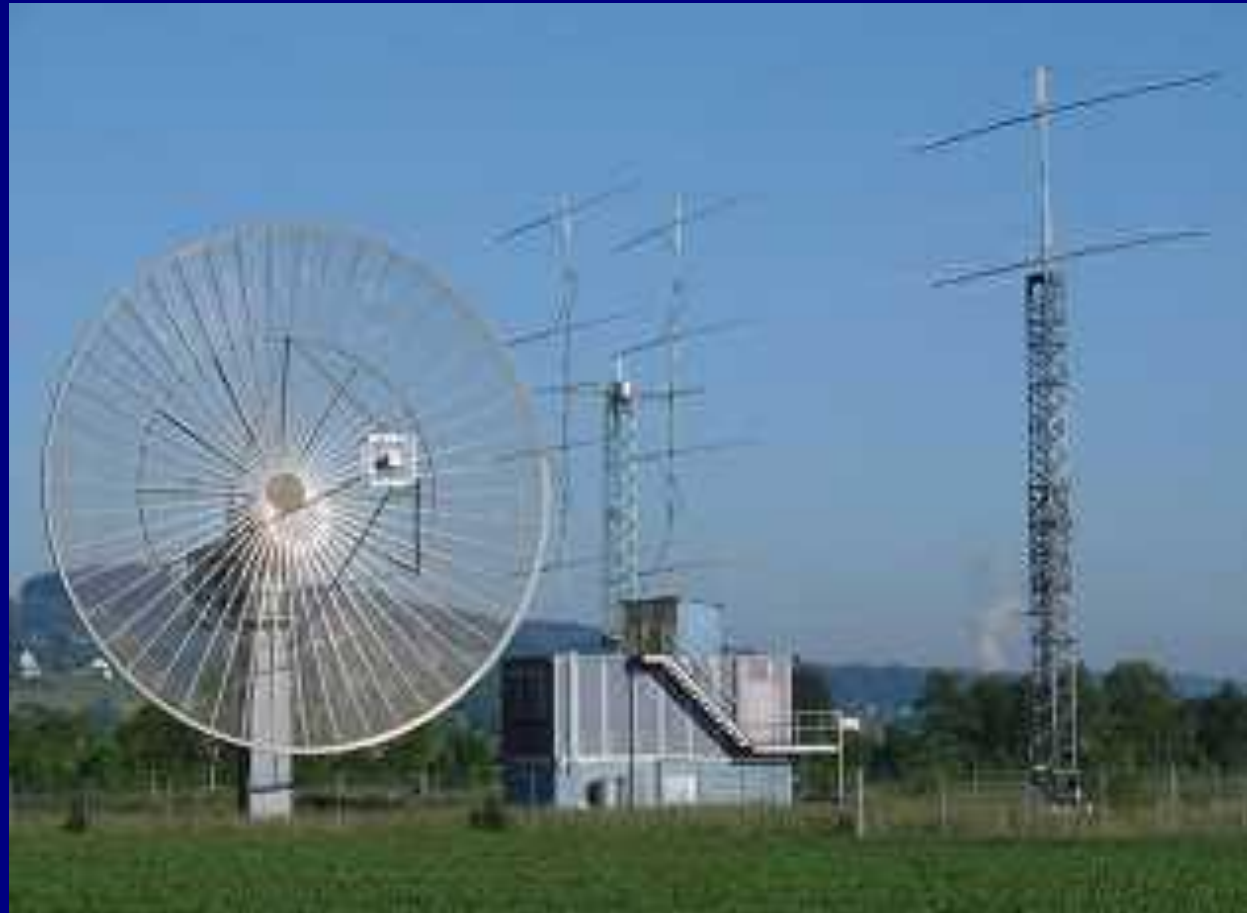
HB9Q Club – 15m Dish (70cm, 23cm, 13cm), 8 x 19 el. Yagis (2m), 11 el. Yagi (6M)
