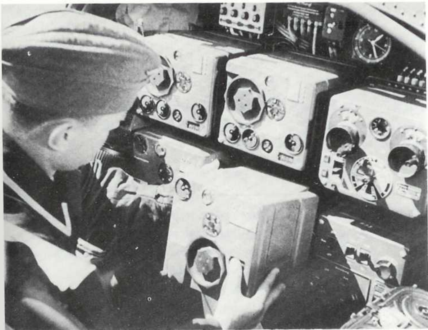
A typical radio installation in a night bomber (Ju88) c. 1940. A signals mechanic is plugging in a replacement transmitter. This FuG10 equipment was modular and extremely advanced, all the connections being made automatically, thus avoiding vulnerable plugs and cables.
